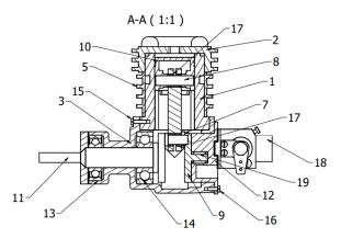
Fig. 6. Cross-section of a typical two-stroke glow engine, fragment of the assembly drawing [12]
