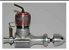
Fig. 3. Polish self-ignition engine "Jaskółka" with a capacity of 2.5 cm<sup>3</sup> [26]
